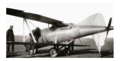
One of the most unorthodox single-seat fighters built during WWI, was the extraordinary pusher biplane with canard configuration.
