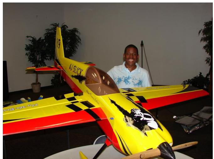
Newest TCRC member Dan Collier had a giant-scale 3D Slick 540 ARF. This plane was done in yellow and red with graphics Dan designed himself. He said it took him one week to assemble the 540 which was powered with an electric Hacker 80-10, which is equivalent to an 80 cc gas engine. The wingspan was 80 + inches and it weighed in at 23 pounds. Dan has 11 flights on the plane and says it has great flying characteristics.
