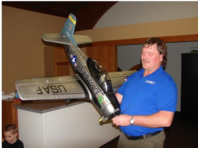
Gerry Dunne had a nice looking foam T-28 ARF done in silver with black trim. The detail on the plane was very nice. It had a 55-inch wingspan and weighed in at 84 ounces. The manufacturer was JR and it was powered with a 4850 500 KV 700 watt motor. The battery was a 4-cell lipo. Gerry said it flew like a 'big trainer.'
