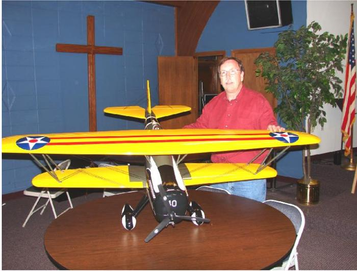
Steve Meyer had a very nice Great Planes ARF of a Curtiss P6E. This biplane was done in Army trainer colors of black fuselage with yellow wings, covered with Monokote. The plane was powered with a Saito 180 4-stroke engine and had a 76-inch wingspan, making it IMAA legal. It weighed 14 pounds and had not flown yet.
