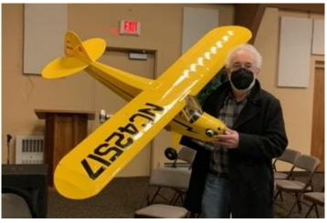
Pedro Restrepo had a Real Planes Piper J-3 Cub for S&T. This was a clipped wing model with a 61.5-inch wingspan and weighed in at 6.5 pounds. It was done in Ultrakote in conventional J-3 Cub yellow with black lightning bolt on the fuse. Pedro got the partially-built lane from Bob Breisemeister and he completed the construction. It was powered by an ASP 52 engine. The date of the maiden flight has yet to be determined, but will be soon.
