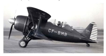
Aerodynamically probably the most elegant fighter biplane ever created, the single-seat fighter was designed by Michael Gregor. It was an all-metal single-bay staggered wing biplane with a semi-monocoque fuselage, flush-riveted, with metal stressed skinning, hydraulically retractable landing gear, and a sliding cockpit canopy.
