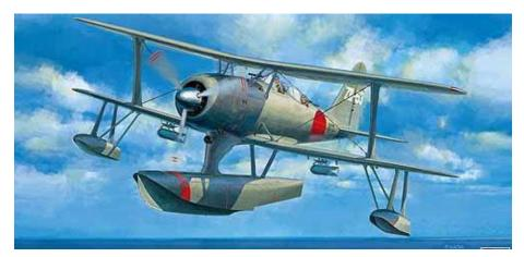
In 1934, Japan, probably anticipating its attack on the U.S.A., ordered a ship launched observation biplane. The design program was assigned to Joji Hattory. Her produced a very neat plane. It featured an all-metal oval fuselage, and all-metal wings. To keep it aerodynamic, he restricted the interplane struts and limited the rat's nest of flying wires. It was engine with an 820 horsepower radial.
