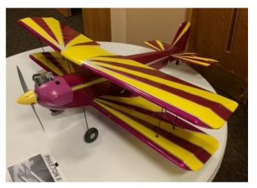
Ken Weddell had a Phaeton II built from a Balsa USA kit. He purchased this plane at the 2019 TCRC auction. It was done in conventional red and yellow sunrays on the wing with a red fuse. The plane had a 52-inch wingspan and weighed in at 6-pounds. It was powered with an OS 70 Surpass 4-stroke engine. He changed out the included servos for Hitec 81-MG's. The Phaeton has not had its maiden flight as yet.
