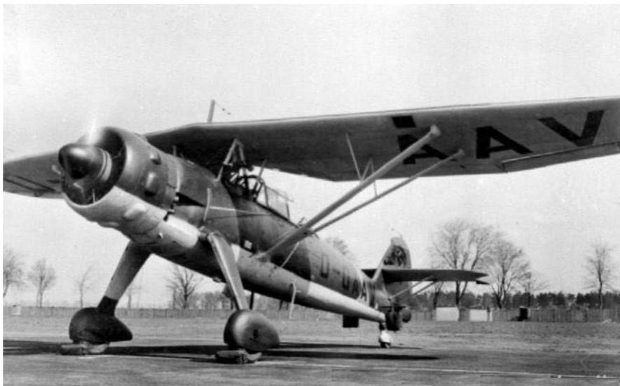
From an earlier similar airplane, the HS-122, the Henschel Company derived the 126, 2-seat econ plane with new wings, hydraulic landing gear, and with a new canopy to cover the pilot. The airframe was improved for the fitting of a new engine, with more power.
