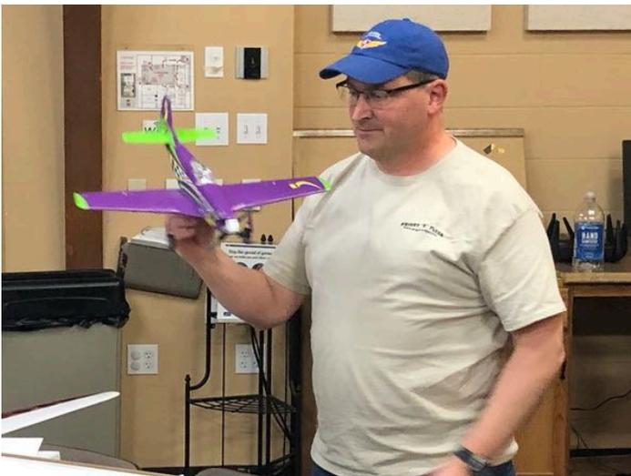
Darryl Volk had a tiny UMX P-51D Voodoo manufactured by E-Flite. (See photo at bottom left.) This plane had a 19.4-inch wingspan and weighed only 4 ounces. It was a lavender color and was powered with an electric 2150 kv outrunner motor. Darryl said that he has flown the plane and it is fast and agile.
