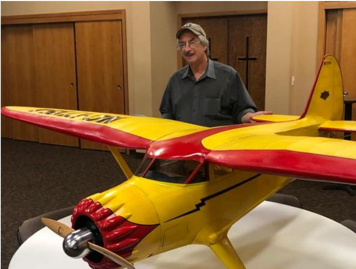
Mark Wolf had a giant-scale Stinson Reliant (SR-9) which was constructed from a Top Flite kit. The plane had a 100-inch wingspan and weighed in at 24.9 pounds. It was done in yellow with red trim on the cowl and the leading edges. For power it had an RCGF 40 Twin. Mark said he had to rework the firewall to allow for the installation of the twin engine. He said he has put the maiden flight on the Stinson.
