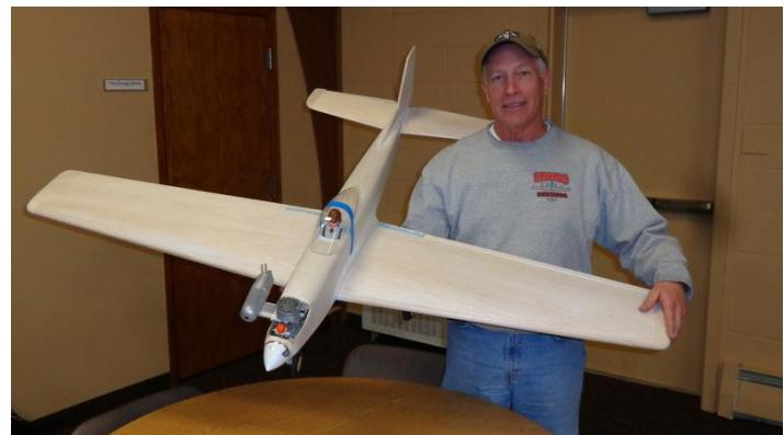
Mr. Giant-Scale, Chris O'Connor had a rare smaller airship at the meeting. This was a Tiger Tail, designed by Ron Chidgey and built from a Eureka Aircraft short kit. The plane had a 66-inch wingspan and weighed in at 6.5 pounds, less the finish and the radio equipment. The power plant was a glow OS 61 FX swinging an 11x8 prop. Chris plans on using Stits paint system and the plane will be done in 70's pattern-style markings. J
