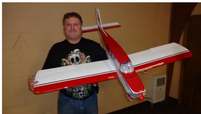
Mr. Electric, Gerry Dunne, had a 40-size electric Cherokee. This plane was a Great Planes ARF and was done in red and white Monokote. It had a 60-inch wingspan and weighed in at 6.5 pounds. The motor was a Turnigy 5055 and was powered with a 4,000 mah 5-cell lipo. It also had flaps. As of the meeting, the maiden flight had yet to be flown.
