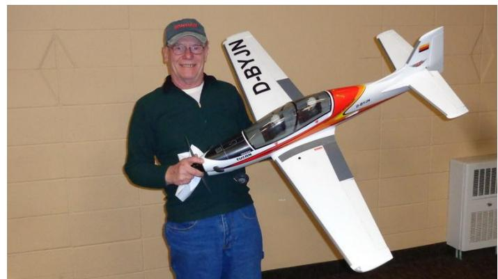
Joe Neidermayer had a nifty looking Tucan ARF by Multiplex. This plane had white wings and fuse with gray and red trim. It had a 51-inch wingspan and weighed in at 3-1/2 pounds. It was powered with a Turnigy electric motor with a pair of 2,000 mah 3-cell lipos. Joe had added retracts to the plane from Hobby King. He has already had flights on the plane and said it flew very well with no trim adjustments necessary. He felt the plane was very acrobatic.
