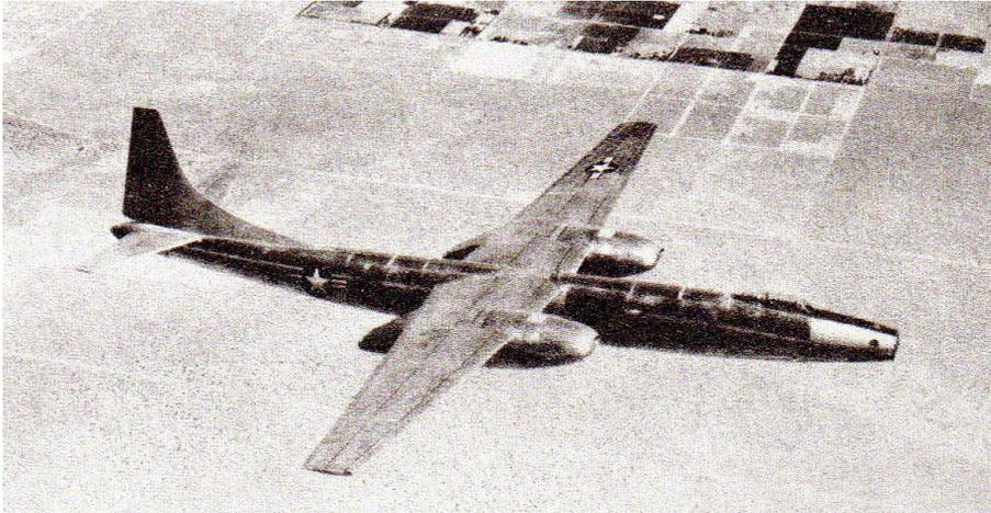
For a 1944 jet bomber competition, Convair offered their very graceful "Model 109" slated to be powered by the new J-35 engine, with 4,000 pounds of thrust. Convair offered two prototypes, but their funds were then divided between two separate projects, and the design on the 109 suffered. The single aircraft completed was first flown April 2, 1947. Its very slim exterior belied its 48,000 pound empty weight. The wings used the Davis airfoil, and an expected bomb load of 22,000 pounds.
