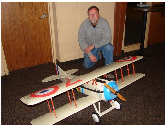
ed with a plastic-like Monokote. It was done in a tan and had large roundels on the wings and fuse. It had a wingspan of 68 inches and weighed in at 14 pounds. The power plant was a Zenoah G-26 and swung an 18x6 prop. Steve said the plane has yet to have its maiden flight.
