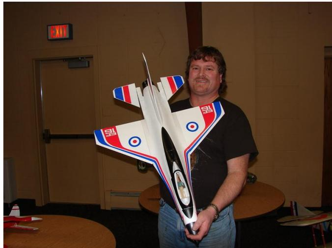
Gerry also had another electric ARF at the meeting. This one was an F-16 manufactured by Phase 3. It was done in white with red and blue trim on the wings and stab. The power plant was a ducted fan using a HET 2W motor and a 2650 mah 3-cell lipo.
