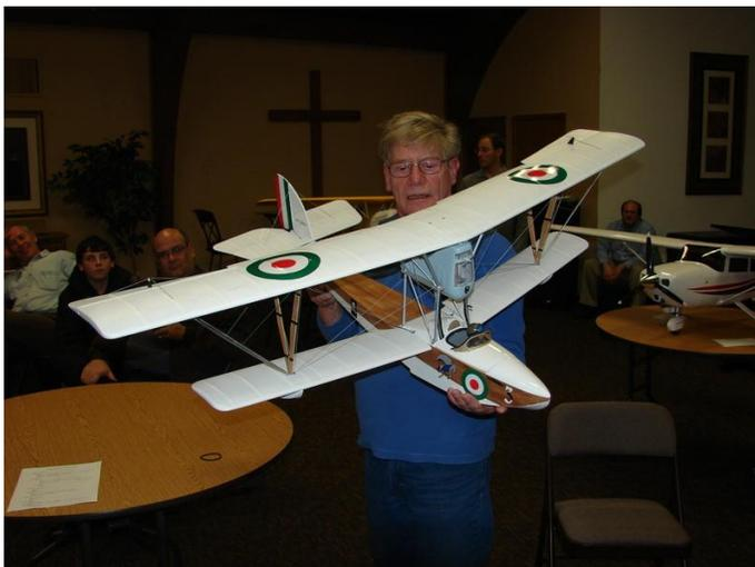
Joe also had a Macchi M5 manufactured by Park Flyer Plastics. Joe called it a 'short kit'. This biplane had white wings and fuse of Koverall but he had added a wood covering on the fuse. The wings had a cable strut system for strength. The wingspan was 51 inches and total weight was 2.6 pounds. Motor was a 2822 1200 KV pusher.
