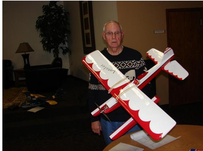
Conrad Naegele had a nifty looking electric Lorelei on floats. He built this plane from plans and was covered with Ultrakote. The wings were white with red scallops on the leading edge and the fuse was red and white. The wingspan was 36 inches and fully loaded it weighed in at 20-1/2 ounces. The motor was a BP 2112 and the battery was a 1320 mah 3-cell lipo. As of the meeting, Conrad had not put the maiden flight on this float plane.
